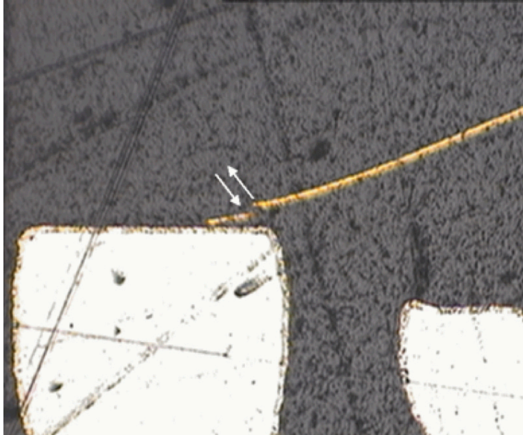
Figure 4: This is a bright-field optical image showing a broken bond wire at the wedge bond. [96X ref. 245AO_6]
