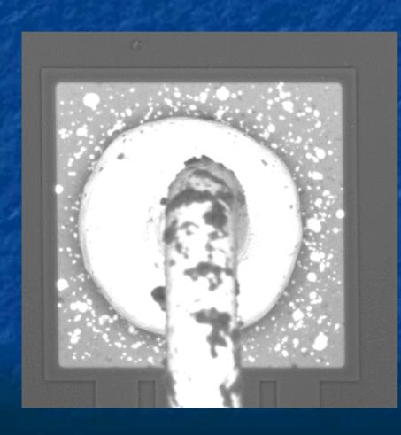
Bright spots are Ti-W barrier layer where Al is missing
