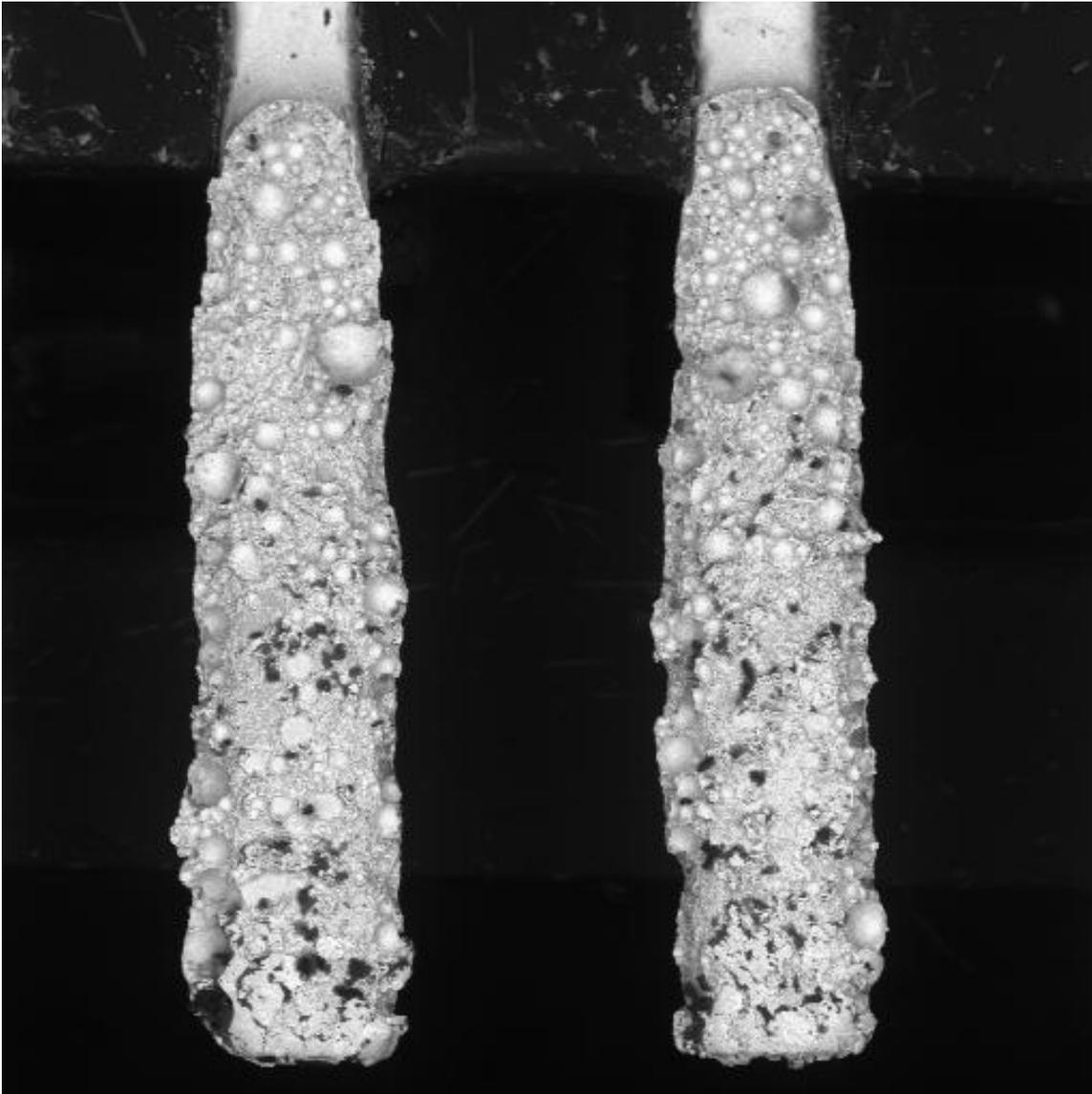
Figure 3: [Ref. IFN 897A\_1, BSE SEM image, 94X] This is a BSE SEM image of the fracture surfaces of failed connector solder joints. There is severe voiding and flux entrapment (dark material) associated with the fracture surface.
