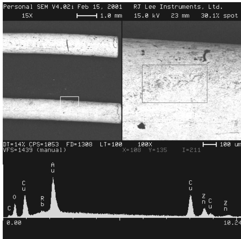
Fig. 5 – Elemental spectrum and BSE SEM images of gold-plated brass leads with no diffusion barrier [ref. SLI-475]. The elemental spectrum shows that there is oxidized copper and zinc on the lead surface, which explains the solderability problems reported on the device leads.
