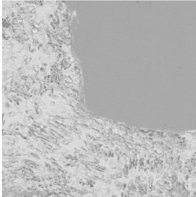
Fig. 3a – [994X, ref. SLI-1110]. Iron (Fe) from this Alloy 42 IC lead appears to have a significant impact on the microstructure of the bulk SAC solder alloy.
