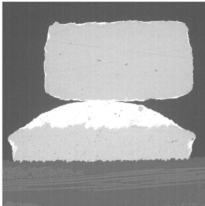
Fig. 2 – Solderability problem on Fe-Ni alloy IC lead with no apparent Ni-barrier [243X BSE SEM] [ref. SLI-168]. The solder from the pad did not wet the lead.
