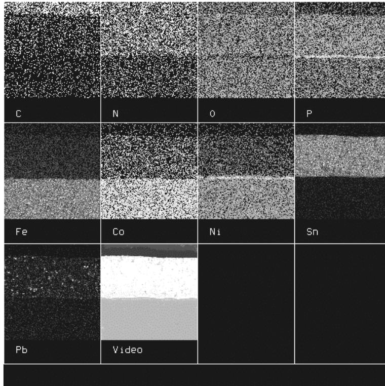
Fig. 4 - This is an elemental dot map of the lead finish/base metal. There is an electroless nickel (Ni-P) layer between the Kovar base metal (Fe-Ni-Co) and the tin-lead plating. [284X, ref. SLI-1076].
