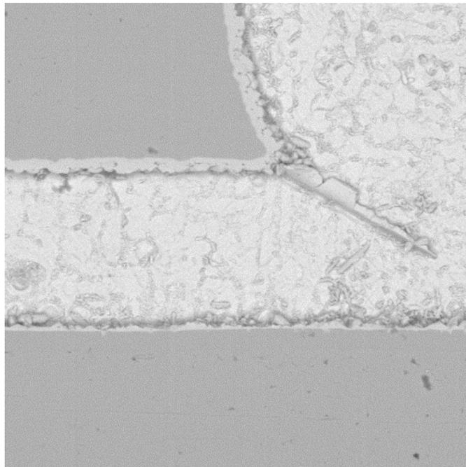
Fig. 3b – [796X, ref. SLI-1110]. This is considered a “normal” microstructure (compare with Fig. 3a) for lead-free 305 SAC alloy. The lead (top-left) is phosphor-bronze. The PWB mounting pad (bottom) is ENIG-finished copper.
