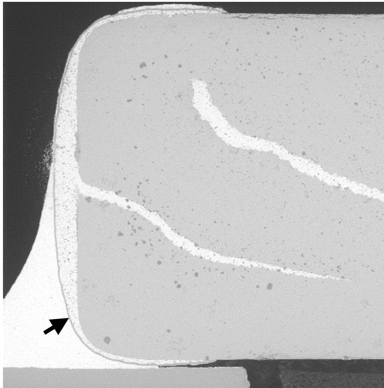
Fig. 1 – Nickel barrier layer on soldered MLCC termination [100X BSE SEM image].
